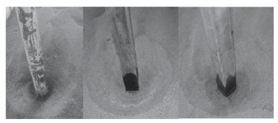
Figure 7: Resultant Scour hole shapes for three different types of pier models used in the experiments
