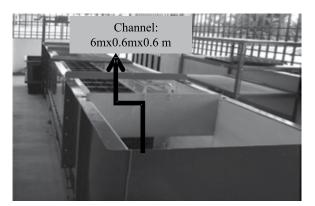
Figure 2: Rectangular Open Channel in Physical Modeling Laboratory of REDAC, USM Malaysia
