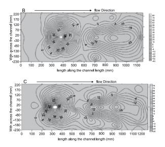
Figure 12: Contour maps for the experimental data collected in Malaysia for 5cm pier model where (A) Circular pier model, B) Square pier model, C) Sharp edged pier mode.
