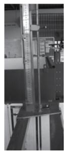
**Figure 4: Vertical Point Gauge**
