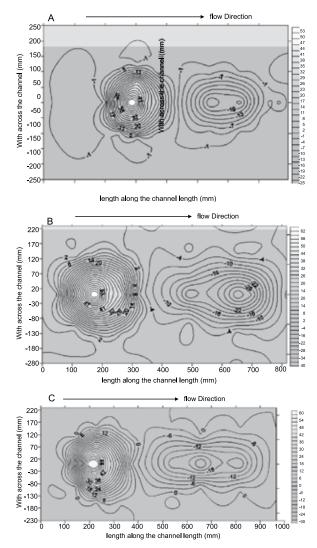
Figure 11: Contour maps for the experimental data collected in Malaysia for 4cm pier model where (A) Circular pier model, B) Square pier model, C) Sharp edged pier model
