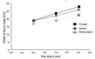
Figure 10: Variation of Width of Scour Hole with variation in Pier size and Shape
