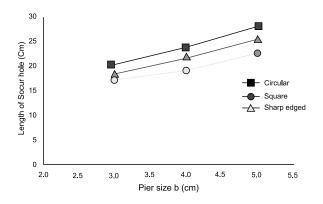
Figure 9: Variation of Length of Scour Hole with variation in Pier size and Shape
