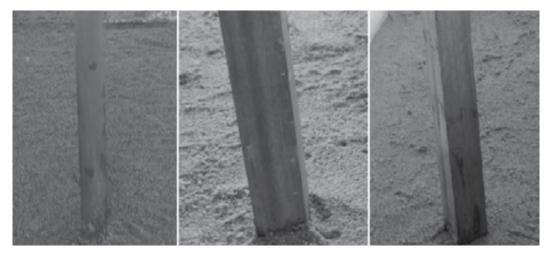
Figure 5: Three pier models used in this study (1. Circular 2. Square 3. Sharp edged)
